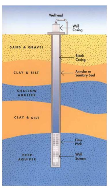
Where the hole intersects the best water producing layers, the driller installs the well casing with thick cuts or perforations. This portion of the well is called the well screen. The well screen allows water to pass into the casing but keeps out sand and gravel. Where the hole intersects layers of clay or fine silt (layers that don't typically produce significant quantities of water), the driller installs un-perforated pipe called blank casing.
